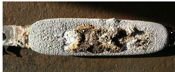
Sacrificial anode on a boat hull. Photograph by Zwergelstern, distributed under a CC BY-SA 3.0 license.
